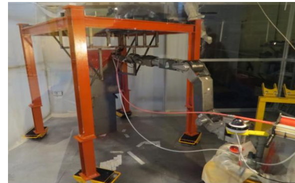
Mock-up with remote controlled arm with spraying nozzle implemented
