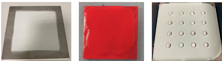
Stainless steel plate with alumina particles deposit (left), with 100% coverage of RTV FA 878 (center) and 90% coverage of RTV FA 873 (right)
