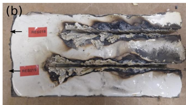
Pictures of the tests: three cuts with the RTV FA 873, 2 cuts with Epoxyguard and 1 cuts with RTV FA FA. Trace of calcination is visible on Epoxyguard
