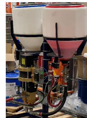
View of the "Matrasur" spraying machine. The coating RTV FA 878 is composed of two components that are mixed together just before the spraying/injection
