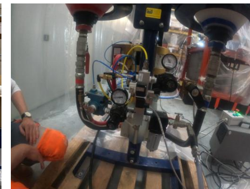
View of the "Matrasur" spraying machine. The coating RTV FA 878 is composed of two components that are mixed together just before the spraying/injection
