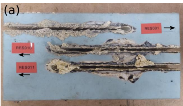
Pictures of the tests: three cuts with the RTV FA 873, 2 cuts with Epoxyguard and 1 cuts with RTV FA FA. Trace of calcination is visible on Epoxyguard
