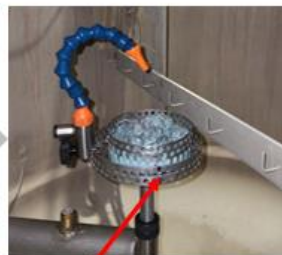
Implementation of coated sample with RTV FA 873 resin inside TOSQAN vessel
