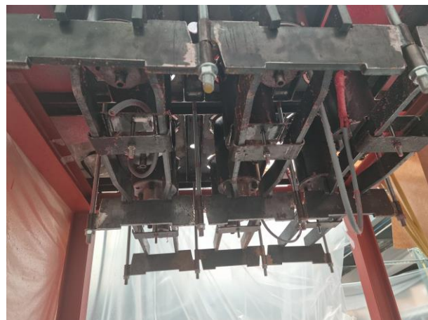
Pictures illustrate the robotic arm is able to properly cover vertical and horizontal flat metallic parts, the cylinders and the screw of the CRD bottom
