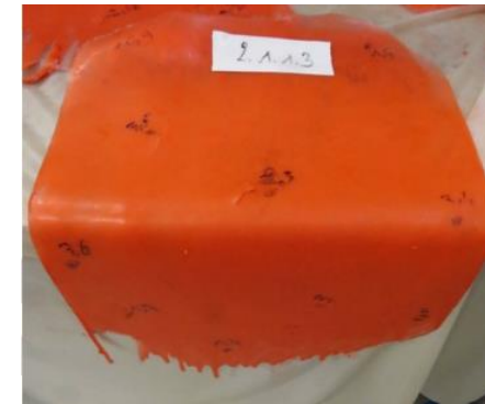
Coating removed from mock-up for thickness measurement
