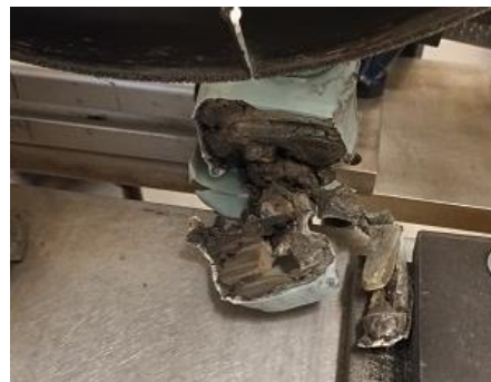
Simulant of corium after a cutting by wheel grind without coat (left), with RTV FA 878 coat (middle) and 873 (right)
