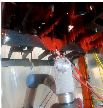
Pictures illustrate the robotic arm is able to properly cover vertical and horizontal flat metallic parts, the cylinders and the screw of the CRD bottom
