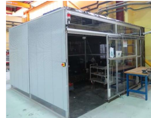
Overview of the test enclosure, meant to be representative of a part of the pedestal, under the CRD-H. Picture on the right shows it is possible to darken the walls with curtains
