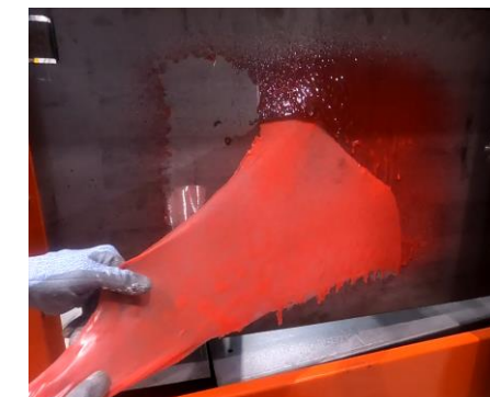
Easily peeling after coating
