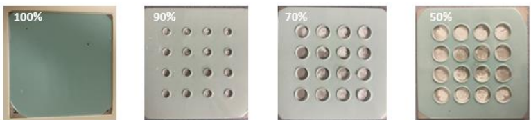
Example of stainless steel plates coated with RTV FA 73 resin. Partial coverage is realized as the above.
