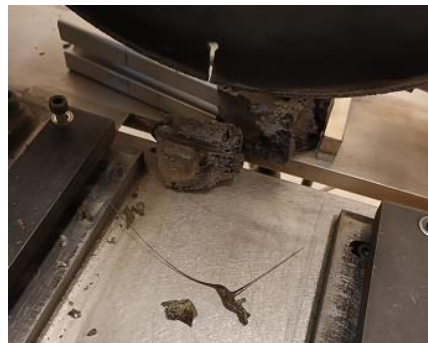
Simulant of corium after a cutting by wheel grind without coat (left), with RTV FA 878 coat (middle) and 873 (right)
