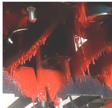
Pictures illustrate the robotic arm is able to properly cover vertical and horizontal flat metallic parts, the cylinders and the screw of the CRD bottom
