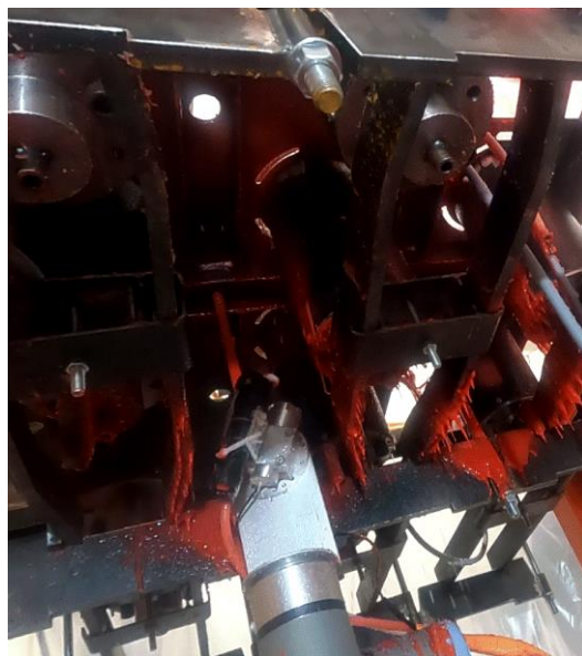
Pictures illustrate the robotic arm was able to spray coating between the CRD-H and that all the surfaces are correctly coated with a 2 mm layer.
