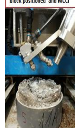
NELC-A configuration inside DELIA Vessel with sample block positioned and MCCI
