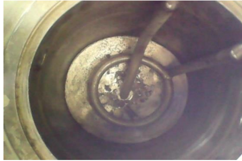
General view of cutting box for in-water cutting (with bubbling system)
